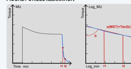
Stress Relaxation test consists of determining the decay of the Mooney torque immediately after the determination of the Mooney viscosity. After abruptly stopping ISO 289-4 the rotor at the end of the Mooney viscosity measurement, the decrease in torque is Unit: recorded as a function of time. The rate of Mu/min change of the torque is evaluated over a
