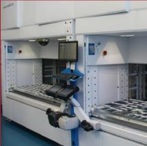
The storage of all production and purchase components is carried out by rotating warehouses to ensure complete traceability of the components and to optimize the shipping times of spare parts
